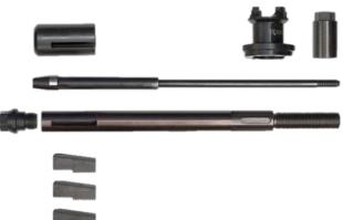
Supplied with 20 mm shaft, one set of jaws to suit plug thread diameter, pilot and gasket seat milling head. Plug size details must be provide by customer with order.
