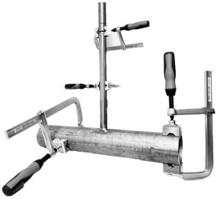
The arms are fabricated from steel which allows a clamping force to meet the requirements for all pipe dimensions within the range of the Clamps. The pads are manufactured from high grade aluminium to ensure rigidity but minimise risk of pipe damage.
