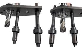
MiniDrill for FinFan applications is delivered with custom locking plate and 2 reaction shafts. Universal construction of the plate allows for locking machine with both shafts on one side to allow to machine the last holes in the row. Plate can be rotated through 180 degrees to accommodatepartition plates, channel heads etc.
