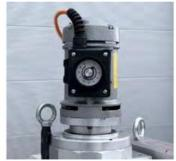
As an alternative, we offer an electric drive for the IMFM-40 and IMFM-60. This electric motor provides similar parameter to the pneumatic version.
