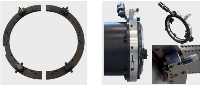
For super heavy applications with thick wall and/or hard alloy pipes, the ORR enhances the axial and linear stability. Manufactured from steel it mounts on the rear of the aluminium ring. It is also equipped with 4 steel location stabilisers to enhance the range and rigidity of the machine for heavy duty applications. The ORR dramatically increases the rigidity when cutting and/or bevelling and also saves time and cost on purchasing clamshells made completely of steel.
