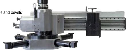
As standard, the IMFM-60 is supplied with a complete toolkit, including tool and inserts, air filter with lubircator and hose connection, required jaws to cover the full range, paper manual and storage/shipping box. Beside standard pneuamtic 4.0Hp drive, we offer a wide range of pneuamtic and electric drives for the IMFM-60.
