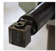
Both machines are equipped with a special jaw set for easy and quick levelling and centring. A special mechanism allows convenient adjustment of the mounting plane relative to the pipe. The built-in self-centring locking system significantly facilitates the coarse setting of the machine.
